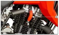
(1) Noise suppressor cap (2) Spark plug
