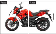
Check the rear mono shock absorber by pushing hard downwards on rear grip while the vehicle is not parked on stand. The suspension action should be smooth and there should be no oil leakage.
