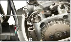
(5) Adjusting screw (6) Valve stem (7) Lock nut
