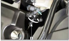
(1) Stop lamp switch (2) Adjusting nut
