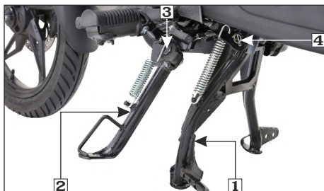
(1) Main stand (2) Side stand (3) Side stand pivot bolt (4) Rear brake pedal/Main stand pivot
