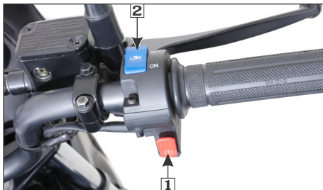
(1) Electric starter switch
